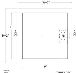
**THREADED RING KEY SHIPPED LOOSE** LATCH CONCEALED TAPE TO BACK OF DOOR HINGE **FOAM INSULATION** FRAME **NEOPRENE** 25/16" **GASKET** (<del>(</del>(**(**)) 1/8" WIDTH (4 SIDES)
